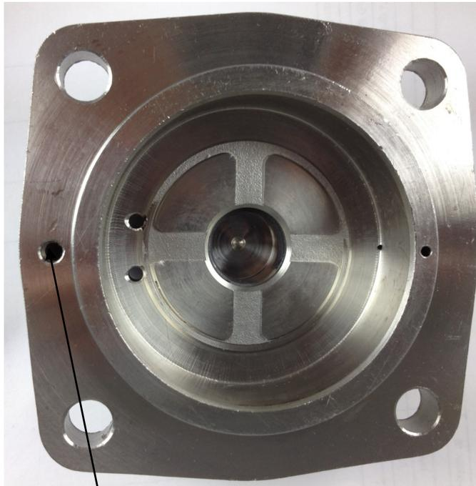
During re-assembling of the valve, make sure the large hole on the top half of the valve lines up with the hole on the bottom half of the valve
